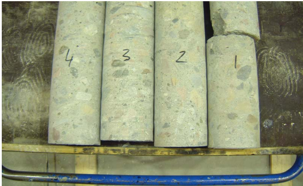
Figure 4:2 Bottom edge of drill cores from test positions up to and including 4 (from left to right)
