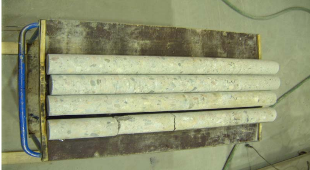
Figure 4:1 Drill cores from test positions up to and including 4 (4 at top)
