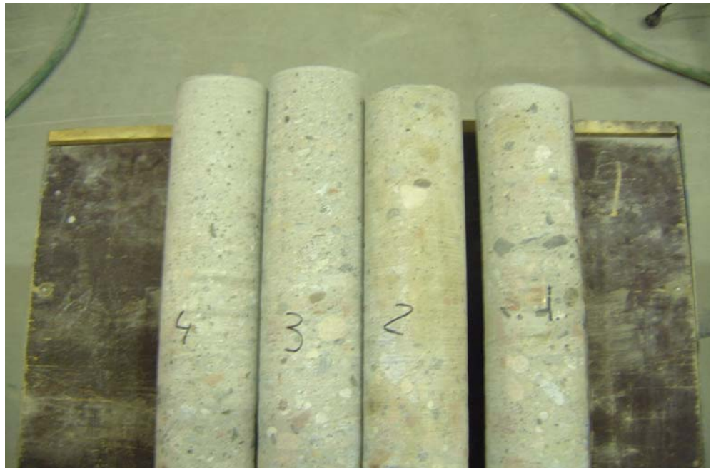
Figure 4:3 Upper edge of drill cores from test positions up to and including 4 (from right to left)
