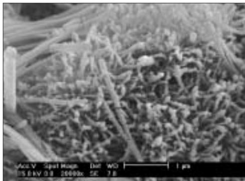
Microphotograph of a cementitious matrix obtained by mixing Keracolor with water
