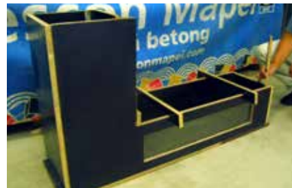
L-box for testing Rescon T ®
