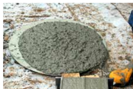
Good workability T-concrete: slump flow > 550 mm
